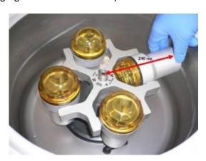
Example: Eppendorf 5702 (4 x 85 round bottom swinging bucket) with a radius of 140 mm. Enter 2000 rcf/G-force and radius of 140 mm into calculator = 3571 round down to 3500 RPM.
