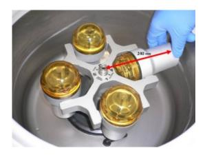
Example: Eppendorf 5702 (4 x 85 round bottom swinging bucket) with a radius of 140 mm. Enter 2000 rcf/G-force and radius of 140 mm into calculator = 3571 round down to 3500 RPM.
